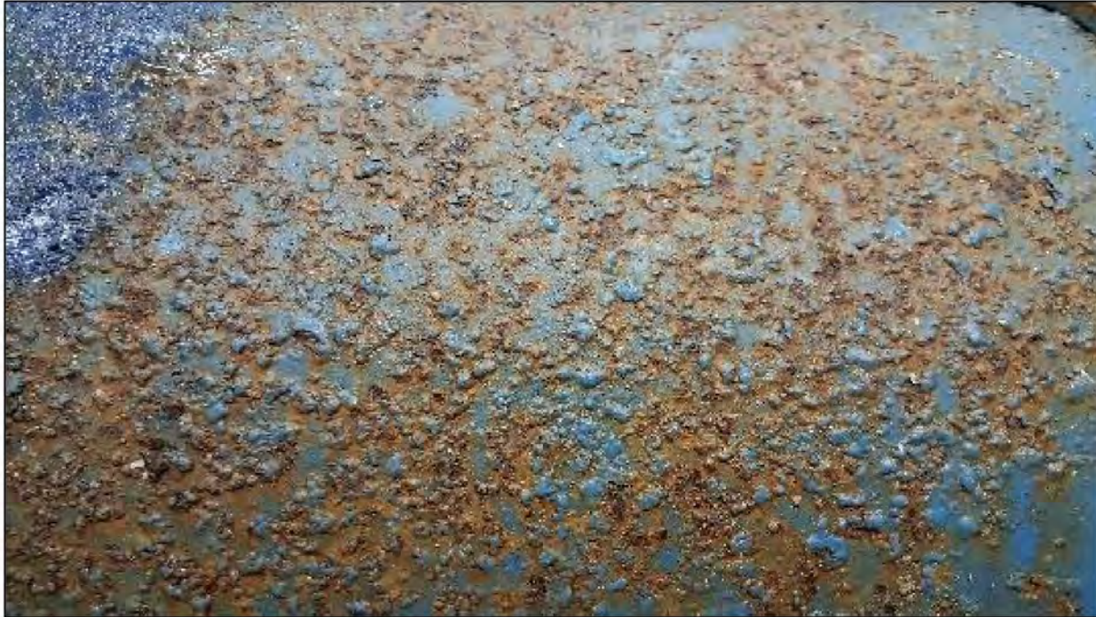
Exhibit 6.10: Close Up Image of Corrosion on Piping
